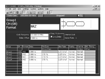
Figure 2-12: Timing window (Data Generator mode)
