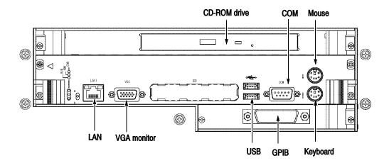
Figure 1-1: Locations of peripheral connectors on rear panel
