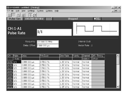
Figure 4-5: Timing window (Pulse Generator mode)
