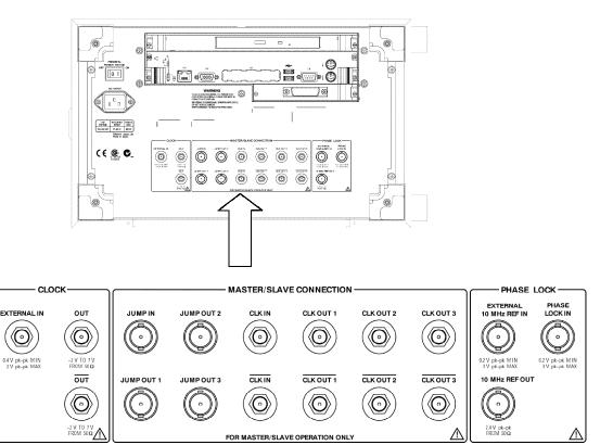
Figure 2-3: Rear panel connectors
