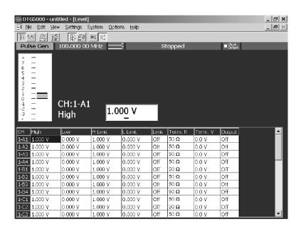
Figure 4-4: Level window (Pulse Generator mode)
