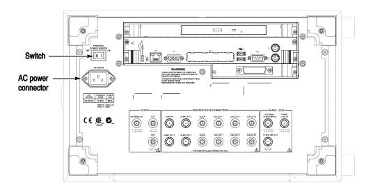
Figure 1-2: Principal power switch and AC power connector
