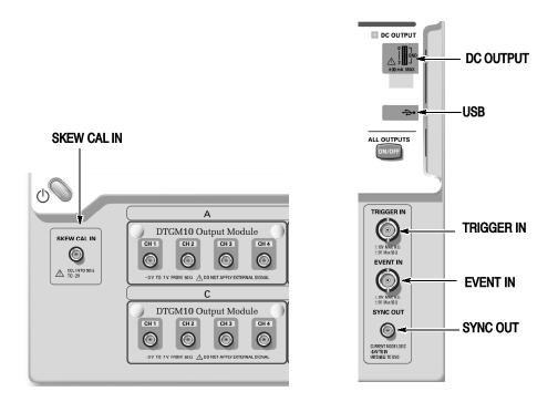
Figure 2-2: Front panel connectors
