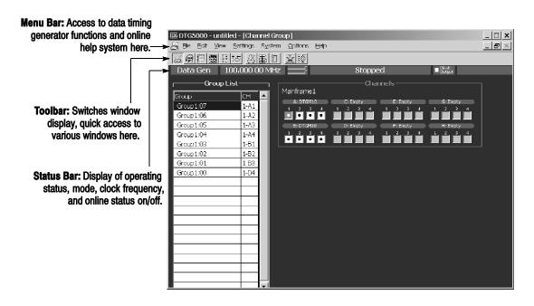
Figure 2-4: Screen elements just after the power on
